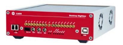
Use of new CAEN electronics-DT5742 12 bit 5 GS/s Switched Capacitor ADC based on DRS4 chip (Paul Scherrer Institute design) to digitize the shape of signal.
