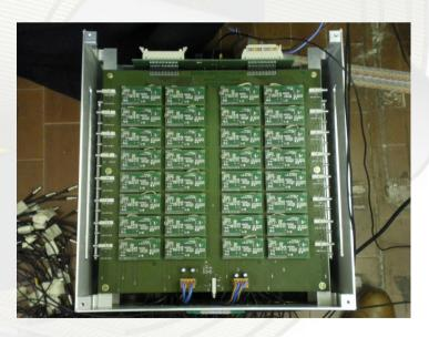
A dedicated preamplifier board has been developed for the experimental set-up. Main Characteristics are:
