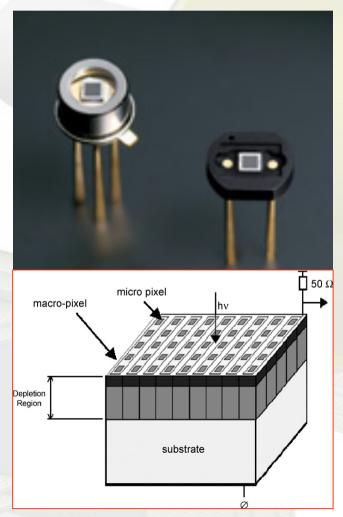
They consist of a P-N junction array working in Geiger mode (micropixel)
