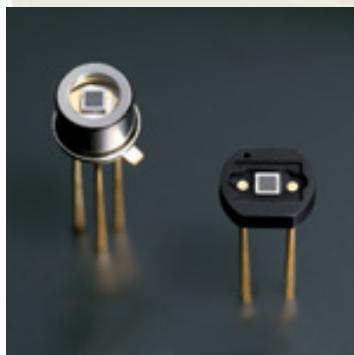
SiPM (HAMAMATSU U50) (400 pixels) Operating voltage \sim 70V
