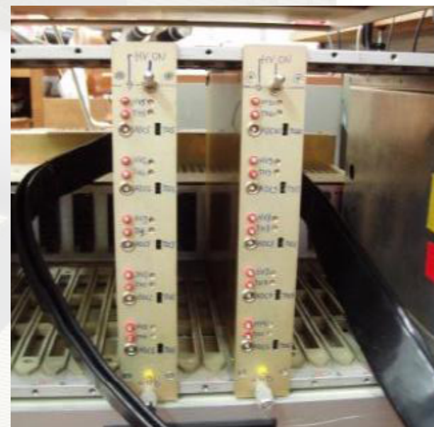
5 Channels HV power supply (stability better than 10 mV)
