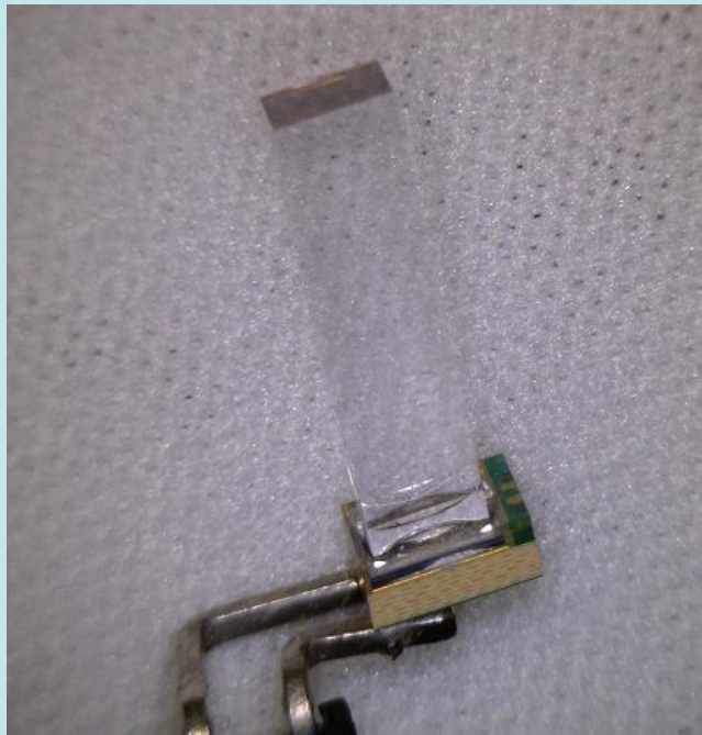
Hamamatsu MPPC coupled to the LYSO crystal
