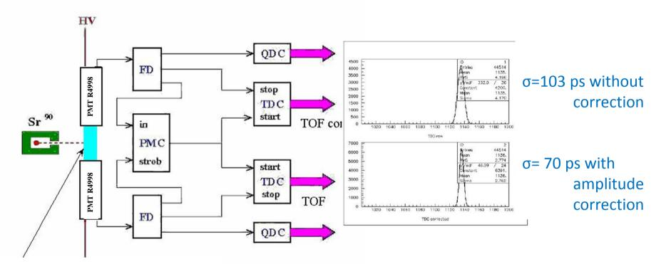
Scintillator B408 20x20x20 mm<sup>3</sup> 2 PMT Hamamatsu 4998
