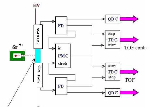
Scintillator B408 3x3x40 mm<sup>3</sup> PMT Hamamatsu 4998 SiPM Hamamatsu S10931-50p  $\sigma$ =147 ps 2 PMT's  $\sigma$ =120 ps PMT + SiPm without correction  $\sigma$ = 65 ps with correction for SiPM
