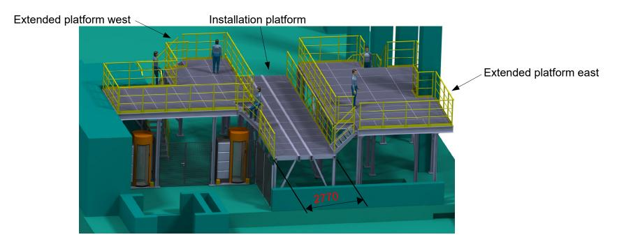
• For that we decided to develop a concept with a movable platform, which allows to make the main mounting and assembling work on the level of the extended platforms and lower it up just for integrating the detectors in the target spectrometer.
